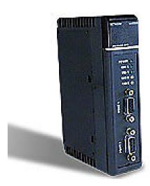
DirectLOGIC DL405 communication module, Modbus RTU, 2 ports, (2) RS-232/RS-422/RS-485 port(s). For use with all DL405 PLCs.
