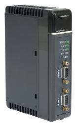
DirectLOGIC DL405 communication module, ASCII, 3 ports, buffered, 128k program memory, 26 MHz maximum switching frequency, (1) RS-232 and (2) RS-232/RS-422/RS-485 port(s). For use with all DL405 PLCs. Commander programming software CD-ROM for Windows included.
