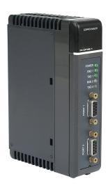
DirectLOGIC DL405 communication module, ASCII, 3 ports, buffered, 128k program memory, 26 MHz maximum switching frequency, (1) RS-232 and (2) RS-232/RS-422/RS-485 port(s). For use with all DL405 PLCs. Commander programming software CD-ROM for Windows included.
