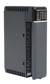
DirectLOGIC DL405 temperature controller module, 4 loop(s), RTD/ thermocouple, jumper selectable inputs, solid state relays. For use with DL405 CPUs.
