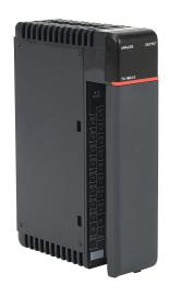
DirectLOGIC DL405 analog output module, 16-channel, voltage, 12-bit, output voltage signal range(s) of 0-5 VDC and 0-10 VDC, external 24 VDC required.
