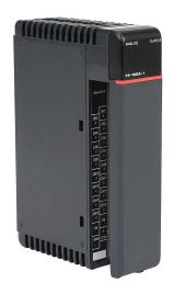
DirectLOGIC DL405 analog output module, 16-channel, current, 12-bit, output current signal range(s) of 4-20 mA, external 24 VDC required.
