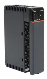
DirectLOGIC DL405 relay output module, 8-point, 12-24 VDC/12-240 VAC, (4) Form A (SPST) no-suppression, (4) Form C (SPDT) no-suppression, 8 isolated common(s), 1 point(s) per common, 5A/point,40A/module. Removable terminal block included.
