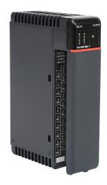
DirectLOGIC DL405 relay output module, 8-point, 12-24 VDC/12-240 VAC, (4) Form A (SPST) no-suppression, (4) Form C (SPDT) no-suppression, 8 isolated common(s), 1 point(s) per common, 10A/point,40A/module. Removable terminal block included.
