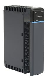
DirectLOGIC DL405 temperature input module, RTD, 8-channel, 16-bit resolution, input RTD type(s): Pt100, JPt100, Cu10, Cu25 and Pt1000.
