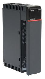
DirectLOGIC DL405 analog output module, 8-channel, voltage, 12-bit, output voltage signal range(s) of 0-5 VDC and 0-10 VDC, external 24 VDC required.
