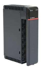
DirectLOGIC DL405 analog output module, 4-channel, voltage, 12-bit, output voltage signal range(s) of 0-5 VDC, 0-10 VDC, +/-5 VDC and +/- 10 VDC, external 24 VDC required.
