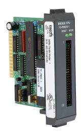
DirectLOGIC DL305 bridge CPU, (1) 50-pin parallel bus port(s), PAMUX.
