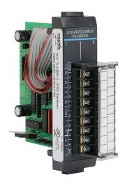
DirectLOGIC DL305 discrete input module, 16-point, 5 VDC/12-24 VDC, sinking/sourcing, fast response, 2 common(s), 8 point(s) per common. Removable terminal block included.
