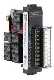
DirectLOGIC DL305 relay output module, 8-point, 12-24 VDC/12-240 VAC, (6) Form A (SPST) no-suppression, (2) Form C (SPDT) no-suppression, 8 isolated common(s), 1 point(s) per common, 5A/point. Removable terminal block included.
