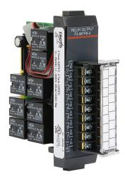
DirectLOGIC DL305 relay output module, 8-point, 12-24 VDC/12-240 VAC, (6) Form A (SPST) no-suppression, (2) Form C (SPDT) no-suppression, 8 isolated common(s), 1 point(s) per common, 5A/point. Removable terminal block included.
