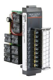
DirectLOGIC DL305 relay output module, 8-point, 12-24 VDC/12-240 VAC, (6) Form A (SPST) no-suppression, (2) Form C (SPDT) no-suppression, 8 isolated common(s), 1 point(s) per common, 10A/point. Removable terminal block included.
