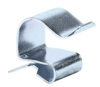
Minerallac flange mount cable clip, package of 100. For use with 1/16 to 3/16in flanges and 0.468-0.562in OD tubing or cable.
