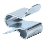
Minerallac flange mount cable clip, package of 100. For use with 1/16 to 3/16in flanges and 0.218-0.281in OD tubing or cable.
