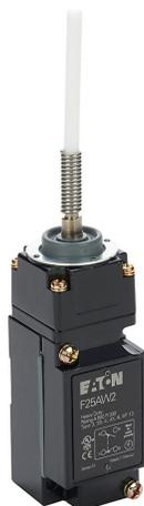
Eaton NEMA limit switch, 360 degree nylon rod, 90-degree adjustable head, (1) N.O./ (1) N.C. contact(s), snap action, 29.4mm x 60mm hole spacing, die-cast zinc, (1) 1/2in NPT cable entry.
