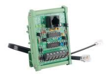
Serial converter, RS-232 (RJ12) to RS-422/485 (6-pin terminal), 5 VDC from PLC nominal input, open frame, DIN rail mount. For use with DL05 and D2-240 CPUs.
