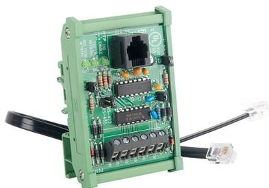
Serial converter, RS-232 (RJ12) to RS-422/485 (6-pin terminal), 5 VDC from PLC nominal input, open frame, DIN rail mount. For use with DL05 and D2-240 CPUs.
