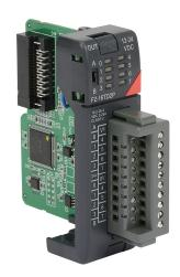
DirectLOGIC DL205 discrete output module, 16-point, 12-24 VDC, sourcing, 1 common(s), 16 point(s) per common, 0.25A/point continuous, overcurrent and overload protection. Removable terminal block included.
