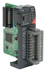
DirectLOGIC DL205 discrete output module, 16-point, 12-24 VDC, sinking, 1 common(s), 16 point(s) per common, 0.25A/point continuous, overcurrent and overload protection. Removable terminal block included.
