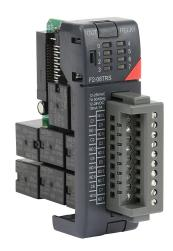
DirectLOGIC DL205 relay output module, 8-point, 12-24 VDC/12-240 VAC, (5) Form A (SPST) no-suppression, (3) Form C (SPDT) no-suppression, 8 isolated common(s), 1 point(s) per common, 7A/point max. Removable terminal block included.
