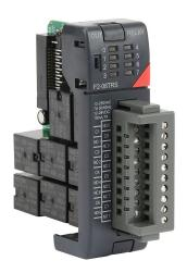
DirectLOGIC DL205 relay output module, 8-point, 12-24 VDC/12-240 VAC, (5) Form A (SPST) no-suppression, (3) Form C (SPDT) no-suppression, 8 isolated common(s), 1 point(s) per common, 7A/point max. Removable terminal block included.
