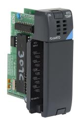
DirectLOGIC DL205 temperature input module, RTD, 4-channel, 16-bit resolution, input RTD type(s): Pt100, JPt100, Cu10, Cu25 and Pt1000.
