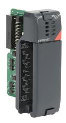
DirectLOGIC DL205 analog output module, 2-channel, voltage, 16-bit, isolated, output voltage signal range(s) of 0-5 VDC and 0-10 VDC, external 24 VDC required.
