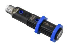
ProSense photoelectric sensor, tubular, threaded, diffuse with background suppression, 50-150mm sensing distance, complementary light-on/dark-on, PNP, teach-in button, 500 Hz switching frequency, 4-pin M12 quick-disconnect.
