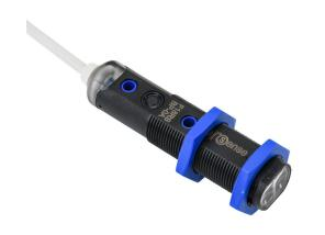
ProSense photoelectric sensor, tubular, threaded, diffuse with background suppression, 50-150mm sensing distance, complementary light-on/dark-on, PNP, teach-in button, 500 Hz switching frequency, 6.5ft/2m cable length, pigtail.
