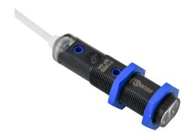
ProSense photoelectric sensor, tubular, threaded, diffuse with background suppression, 50-150mm sensing distance, complementary light-on/dark-on, PNP, teach-in button, 500 Hz switching frequency, 6.5ft/2m cable length, pigtail.
