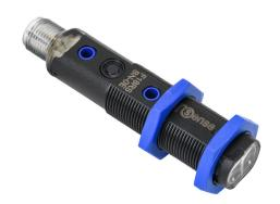
ProSense photoelectric sensor, tubular, threaded, diffuse with background suppression, 50-150mm sensing distance, complementary light-on/dark-on, NPN, teach-in button, 500 Hz switching frequency, 4-pin M12 quick-disconnect.
