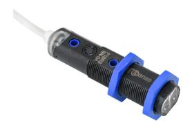
ProSense photoelectric sensor, tubular, threaded, diffuse with background suppression, 50-150mm sensing distance, complementary light-on/dark-on, NPN, teach-in button, 500 Hz switching frequency, 6.5ft/2m cable length, pigtail.
