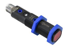
ProSense photoelectric sensor, tubular, threaded, polarized retroreflective, visible red, 0.1-4m sensing distance, complementary light-on/dark-on, PNP, potentiometer, 4-pin M12 quick-disconnect.
