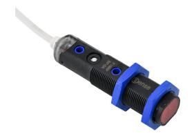
ProSense photoelectric sensor, tubular, threaded, polarized retroreflective, visible red, 0.1-4m sensing distance, complementary light-on/dark-on, PNP, potentiometer, pigtail.
