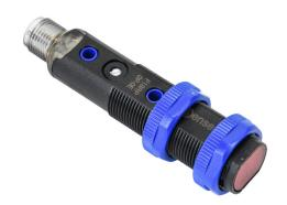
ProSense photoelectric sensor, tubular, threaded, polarized retroreflective, visible red light emission, 0.1-4m sensing distance, selectable light-on/dark-on, PNP, potentiometer, 4-pin M12 quick-disconnect.
