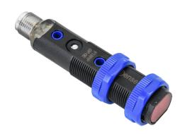
ProSense photoelectric sensor, tubular, threaded, polarized retroreflective, visible red, 0.1-4m sensing distance, selectable light-on/dark-on, PNP, potentiometer, 4-pin M12 quick-disconnect.
