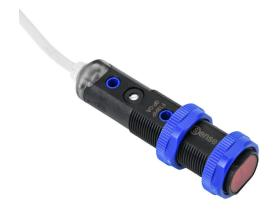
ProSense photoelectric sensor, tubular, threaded, polarized retroreflective, visible red, 0.1-4m sensing distance, selectable light-on/dark-on, PNP, potentiometer, pigtail.
