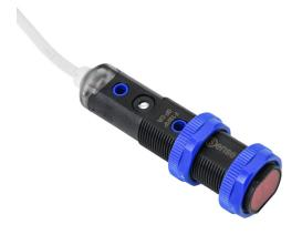
ProSense photoelectric sensor, tubular, threaded, polarized retroreflective, visible red light emission, 0.1-4m sensing distance, selectable light-on/dark-on, PNP, potentiometer, pigtail.
