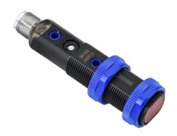
ProSense photoelectric sensor, tubular, threaded, polarized retroreflective, visible red light emission, 0.1-4m sensing distance, selectable light-on/dark-on, NPN, potentiometer, 4-pin M12 quick-disconnect.
