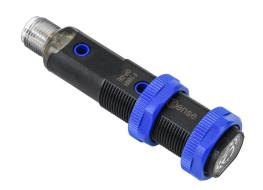
ProSense photoelectric sensor, tubular, threaded, polybutylene terephthalate housing, through-beam receiver, 25m sensing distance, 10-30 VDC operating voltage, selectable light-on/dark-on, PNP, 4-pin M12 quick-disconnect.
