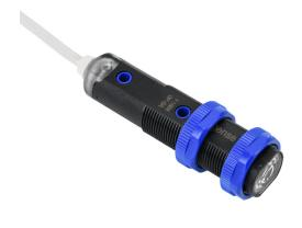
ProSense photoelectric sensor, tubular, threaded, polybutylene terephthalate housing, through-beam receiver, 25m sensing distance, 10-30 VDC operating voltage, selectable light-on/dark-on, PNP, pigtail.
