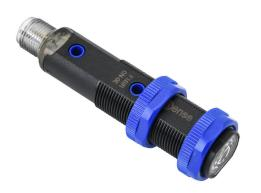
ProSense photoelectric sensor, tubular, threaded, polybutylene terephthalate housing, through-beam receiver, 25m sensing distance, 10-30 VDC operating voltage, selectable light-on/dark-on, NPN, 4-pin M12 quick-disconnect.
