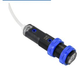
ProSense photoelectric sensor, tubular, threaded, polybutylene terephthalate housing, through-beam receiver, 25m sensing distance, 10-30 VDC operating voltage, selectable light-on/dark-on, NPN, pigtail.
