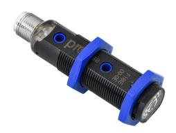
ProSense photoelectric sensor, tubular, threaded, polybutylene terephthalate housing, through-beam emitter, infrared light emission, 25m sensing distance, 10-30 VDC operating voltage, 4-pin M12 quick-disconnect.
