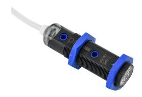
ProSense photoelectric sensor, tubular, threaded, polybutylene terephthalate housing, through-beam emitter, infrared light emission, 25m sensing distance, 10-30 VDC operating voltage, pigtail.
