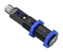
ProSense photoelectric sensor, tubular, threaded, diffuse, infrared, 700mm sensing distance, complementary light-on/dark-on, PNP, potentiometer, 1000 Hz switching frequency, polybutylene terephthalate housing, 4-pin M12 quick-disconnect.
