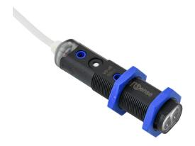
ProSense photoelectric sensor, tubular, threaded, diffuse, infrared light emission, 700mm sensing distance, complementary light-on/dark-on, PNP, potentiometer, 1000 Hz switching frequency, polybutylene terephthalate housing, pigtail.
