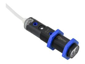
ProSense photoelectric sensor, tubular, threaded, diffuse, infrared, 700mm sensing distance, complementary light-on/dark-on, PNP, potentiometer, 1000 Hz switching frequency, polybutylene terephthalate housing, pigtail.
