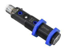
ProSense photoelectric sensor, tubular, threaded, diffuse, infrared, 700mm sensing distance, complementary light-on/dark-on, NPN, potentiometer, 1000 Hz switching frequency, polybutylene terephthalate housing, 4-pin M12 quick-disconnect.
