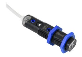
ProSense photoelectric sensor, tubular, threaded, diffuse, infrared, 700mm sensing distance, complementary light-on/dark-on, NPN, potentiometer, 1000 Hz switching frequency, polybutylene terephthalate housing, pigtail.
