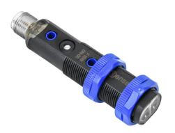
ProSense photoelectric sensor, tubular, threaded, diffuse, infrared light emission, 700mm sensing distance, selectable light-on/darkon, NPN, potentiometer, 500 Hz switching frequency, polybutylene terephthalate housing, 4-pin M12 quick-disconnect.
