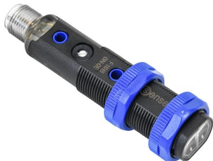
ProSense photoelectric sensor, tubular, threaded, diffuse, infrared light emission, 700mm sensing distance, selectable light-on/dark-on, NPN, potentiometer, 500 Hz switching frequency, polybutylene terephthalate housing, 4-pin M12 quick-disconnect.
