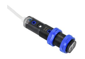
ProSense photoelectric sensor, tubular, threaded, diffuse, infrared, 700mm sensing distance, selectable light-on/dark-on, NPN, potentiometer, 500 Hz switching frequency, polybutylene terephthalate housing, pigtail.
