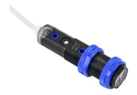
ProSense photoelectric sensor, tubular, threaded, diffuse, infrared light emission, 700mm sensing distance, selectable light-on/dark-on, NPN, potentiometer, 500 Hz switching frequency, polybutylene terephthalate housing, pigtail.
