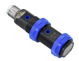
ProSense photoelectric sensor, tubular, threaded, diffuse, infrared light emission, 100mm sensing distance, selectable light-on/dark-on, PNP, 500 Hz switching frequency, polybutylene terephthalate housing, 4-pin M12 quick-disconnect.
