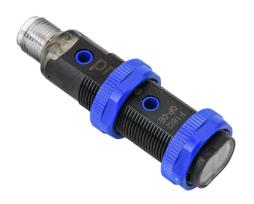
ProSense photoelectric sensor, tubular, threaded, diffuse, infrared, 100mm sensing distance, selectable light-on/dark-on, PNP, 500 Hz switching frequency, polybutylene terephthalate housing, 4-pin M12 quick-disconnect.
