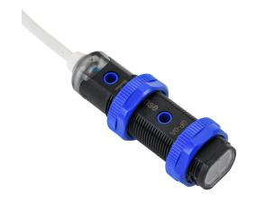
ProSense photoelectric sensor, tubular, threaded, diffuse, infrared, 100mm sensing distance, selectable light-on/dark-on, PNP, 500 Hz switching frequency, polybutylene terephthalate housing, pigtail.
