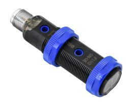
ProSense photoelectric sensor, tubular, threaded, diffuse, infrared, 100mm sensing distance, selectable light-on/dark-on, NPN, 500 Hz switching frequency, polybutylene terephthalate housing, 4-pin M12 quick-disconnect.
