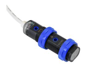
ProSense photoelectric sensor, tubular, threaded, diffuse, infrared, 100mm sensing distance, selectable light-on/dark-on, NPN, 500 Hz switching frequency, polybutylene terephthalate housing, pigtail.
