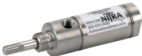
NITRA pneumatic cylinder, all stainless steel non-repairable, 1-1/16in bore, 5/16in rod diameter, 1/2in stroke, double acting, front nose mount.
