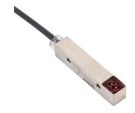
ProSense photoelectric sensor, rectangular, die-cast zinc, diffuse with background suppression, 5-30mm sensing distance, light-on, PNP, 500 Hz switching frequency, 0.6ft/0.2m cable length, 3-pin M8 quick-disconnect.
